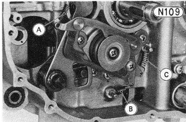
**A. Shift Arm Spring**                      **C. Gear Positioner Spring**
