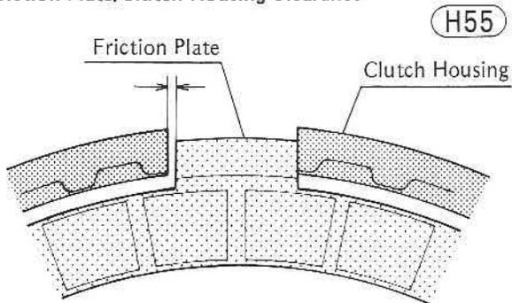
**Table H42 Friction Plate/Clutch Housing Clearance**
