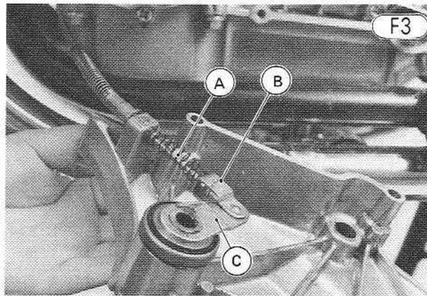
A. Inner Cable      C. Release Lever
