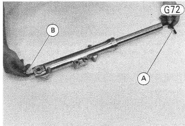
A. Front Fork Cylinder Holder Handle and Adapter
