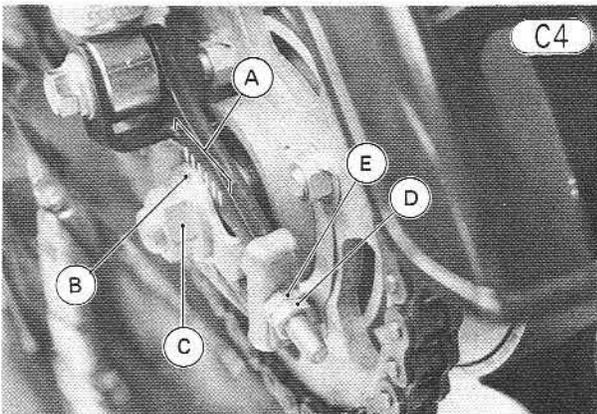
A. Marks B. Notch C. Axle Nut D. Locknut E. Adjusting Nut
