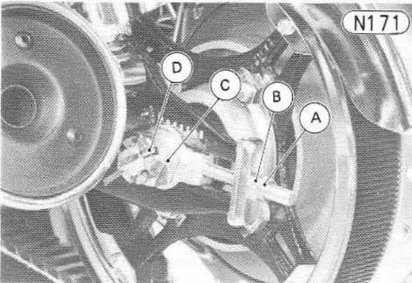
A. Belt Adjuster Locknut      C. Axle Nut
