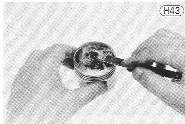
Carbon accumulated in the piston ring grooves can cause the rings to stick. Remove the rings, and clean out any carbon deposits using the end of a broken piston ring or some other suitable tool.
