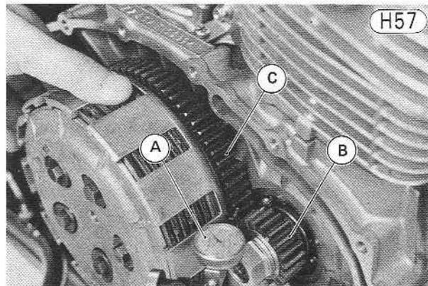
**A. Dial Gauge C. Clutch Housing Gear
