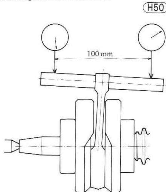
Using the arrangement and arbor shown below, measure the amount that the arbor varies from being parallel with the crankshaft over a 100 mm length of the arbor to determine the amount the connecting rod is twisted.
