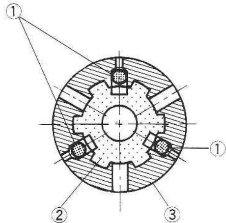
1. Steel Balls                      2. Output Shaft                      3. 5th Gear
