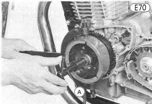
**A. Rotor Puller (57001-1016) and Rotor Puller Adapter (57001-1109)**
