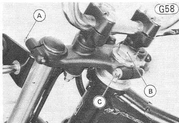
A. Fork Upper Clamp Bolt      C. Head Clamp Bolt
