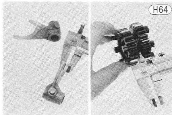
**Shift fork guide pin/shift drum groove wear**
