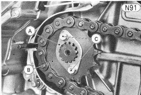
A. Engine Sprocket Holding Plate                      C. Bolts
