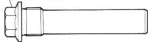
1. One of the 6 mm rocker cover bolts has been discontinued (≠ 2 bolt in Fig. E30 on Pg. 46 and Fig. F61 on Pg. 82). Tightening torque and order for the bolts are not changed.
