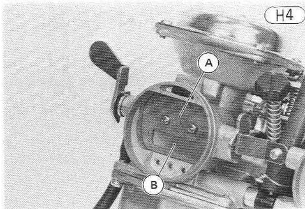
A. Choke Valve      B. Relief Valve
