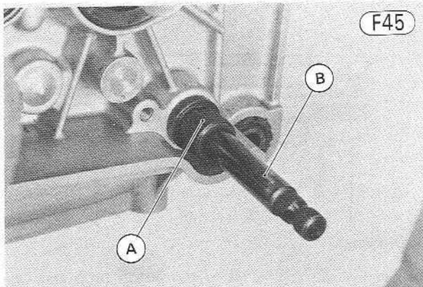
A. Oil Seal Guide (57001-264)      B. Shift Shaft
