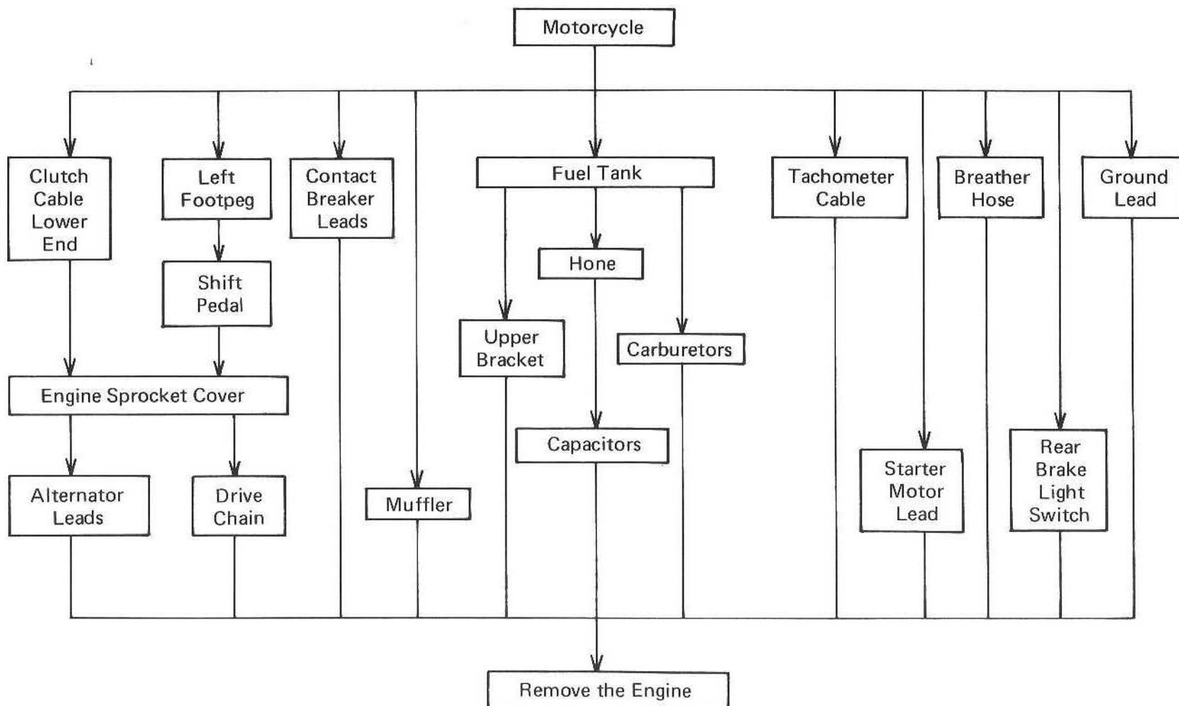
This chart is intended to be aids to proper removal. Select the component you wish to remove and follow the arrows to that point on the chart. Action with a mark ★ requires special tool for removal, installation, disassembly or assembly.
