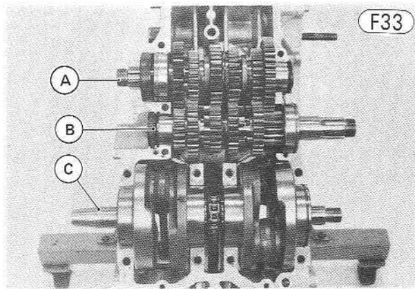
A. Output Shaft Assembly      C. Crankshaft Assembly
