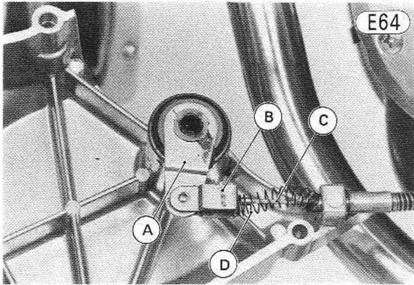
A. Release Lever B. Cotter Pin C. Inner Cable D. Spring
