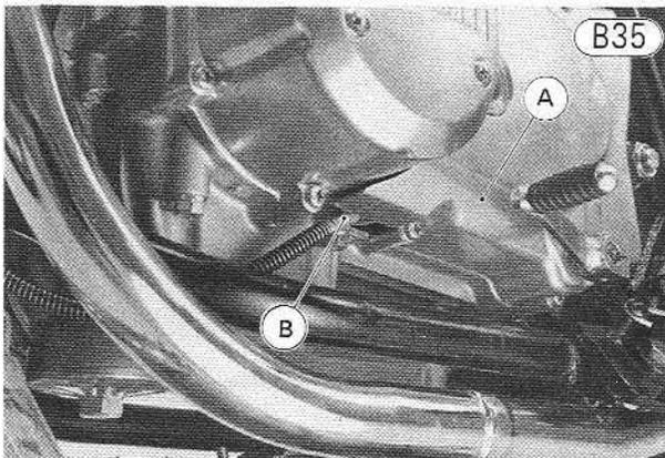
A. Engine Sprocket Cover B. Clutch Outer Cable
