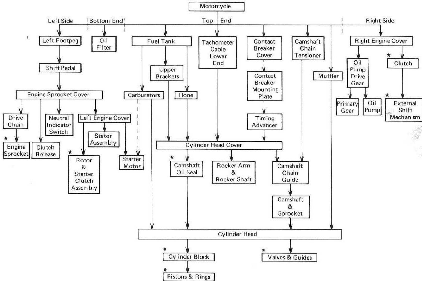
This chart is intended to be aids to proper removal. Select the component you wish to remove and follow the arrows to that point on the chart. Action with a mark \* requires special tool for removal, installation, disassembly or assembly.
