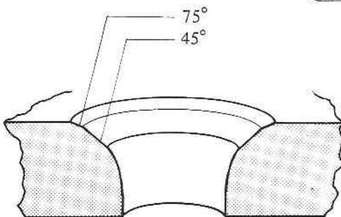
Apply compound to the valve seat, and tap the valve lightly into place while rotating it with a lapper, repeating this until a smooth, matched surface is obtained.
