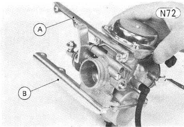
A. Upper Mounting Plate B. Lower Mounting Plate
