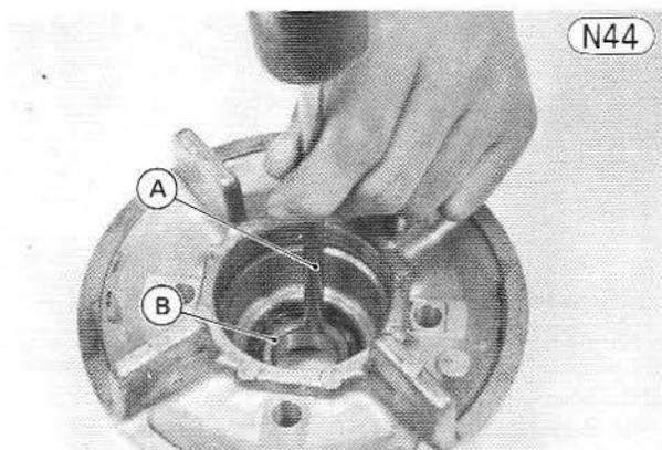
**A. Rod B. Bearing Inner Race****Wheel Coupling Assembly:**
