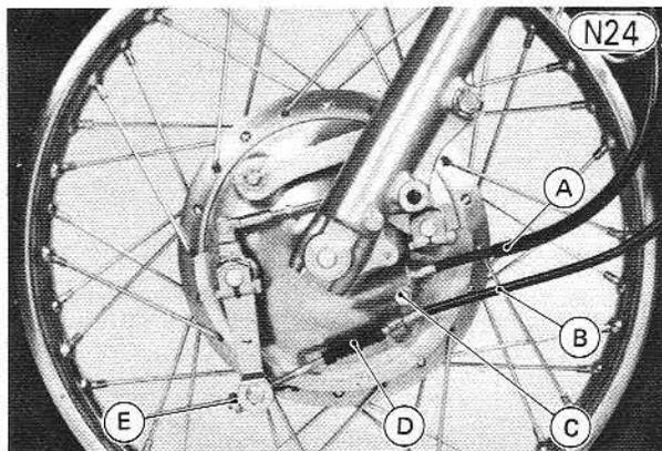
A. Speedometer Cable      D. Dust Cover
