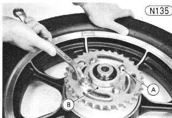
**A. Sprocket Nut    B. Double Washer**
