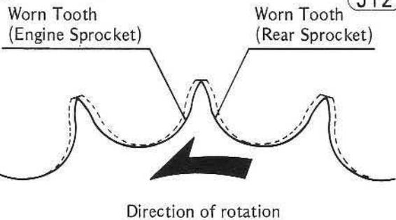
**NOTE:** If a sprocket requires replacement, the chain is probably worn also. Upon replacing a sprocket, inspect the chain.
