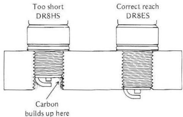
If the plug reach is too short, carbon will build up on the plug hole threads in the cylinder head, causing overheating and making it very difficult to insert the correct spark plug later.
