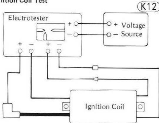
If an Electrotester is not available, the coil can be checked for a broken or badly shorted winding with an ohmmeter. However, an ohmmeter cannot detect layer shorts and shorts resulting from insulation breakdown under high voltage.
