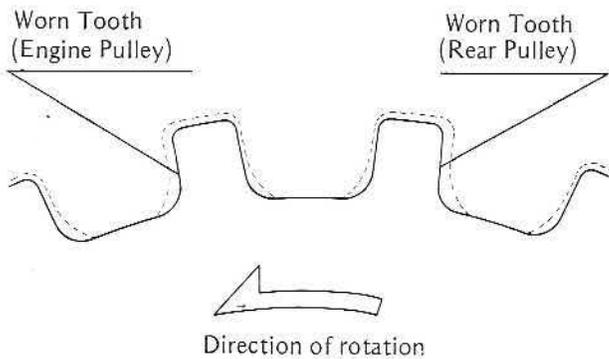
**NOTE:** If the pulley requires replacement, the belt is probably worn. Whenever replacing the pulley, inspect the belt.
