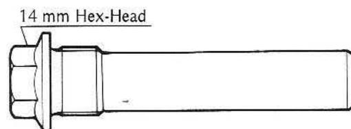
1. One of the 6 mm rocker cover bolts has been discontinued (# 2 bolt in Fig. E30 on Pg. 46 and Fig. F61 on Pg. 82). Tightening torque and order for the bolts are not changed.
