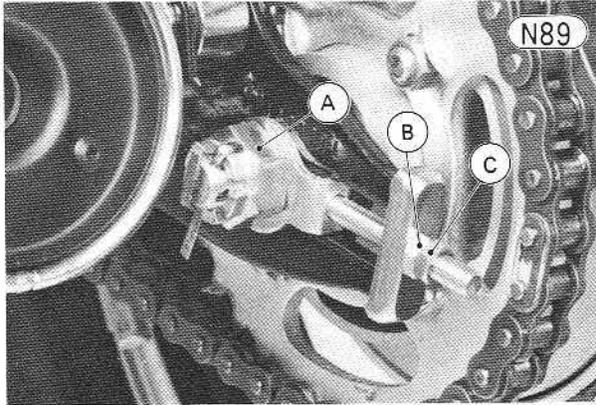
A. Axle Nut                      C. Chain Adjuster Locknut
