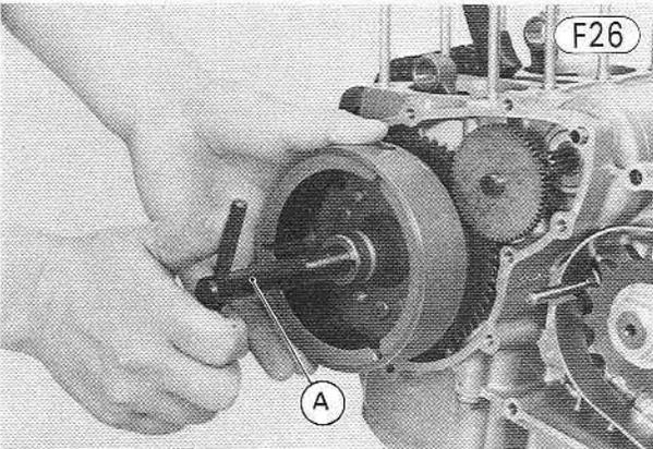
A. Rotor Puller (57001-1016) and Rotor Puller Adapter (57001-1109)
