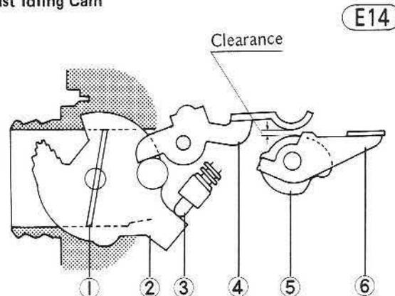
1. Choke Valve 2. Pulley 3. Idle Adjusting Screw 4. Idling Link 5. Idling Cam 6. Choke Lever
