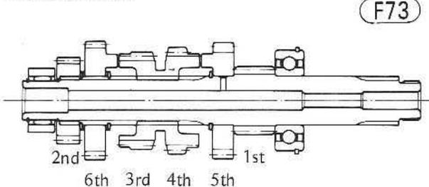
**Output Shaft Disassembly:**
