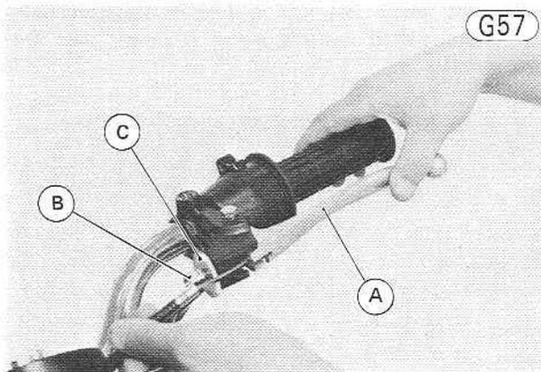
A. Clutch Lever      C. Knurled Locknut
