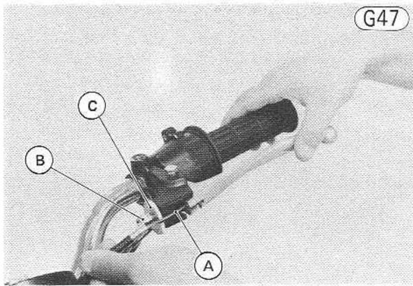
**A. Clutch Inner Cable**      **C. Knurled Locknut**
