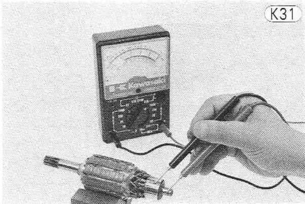
**NOTE:** Even if the foregoing checks show the armature to be good, it may be defective in some manner not readily detectable with an ohmmeter. If all other starter motor and starter motor circuit components check good, but the starter motor still does not turn over or only turns over weakly, replace the starter motor with a new one.
